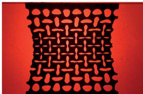
**Fig. 2** Two dimensional silicone rubber sample under vertical compression at  $\varepsilon = 0.25$ . The sample was held between two loose fitting PDMS plates which prevented out of plane buckling. The sidewalls of the initial rectangular sample moved inwards under compression indicating negative Poisson ratio behaviour.
