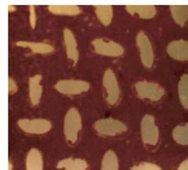
**Fig. 3** Pattern switched state in a jelly which has deformed under its own weight. The initial state was a square lattice of circular holes which switched rapidly to the shown array of orthogonal ellipses when the sample was turned from lying horizontal to standing vertical.
