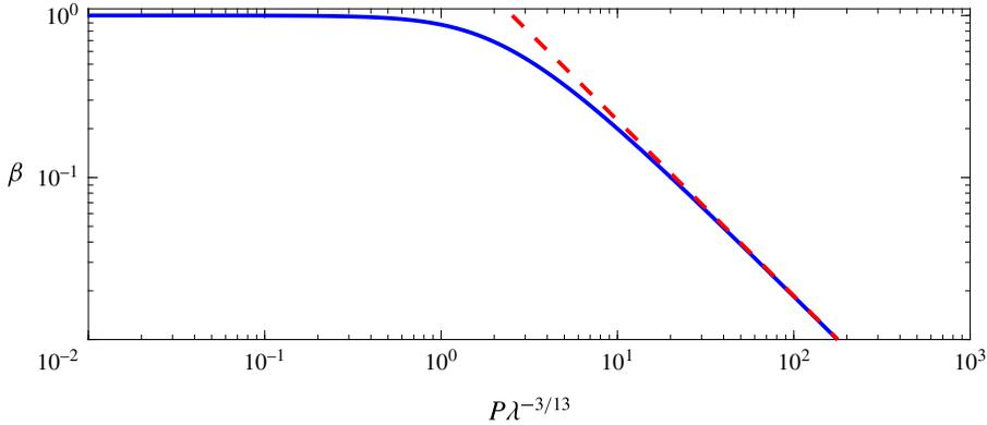
FIGURE 4. (Colour online) The separation point as a function of  $P\lambda^{-3/13}$  from the solution of (3.10), and where the red dashed line indicates the asymptotic limit  $\beta \simeq (2.5315/P\lambda^{-3/13})^{13/12}$ .
