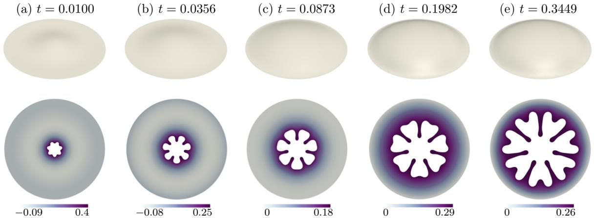
FIG. 5. No wrinkling: time evolution of the air-liquid interface, the corresponding instantaneous pressure fields in the viscous fluid and a perspective view of the sheet deformations (with the transverse displacement increased by a factor of 10) for  $\mathcal{I} = 10^2$ .
