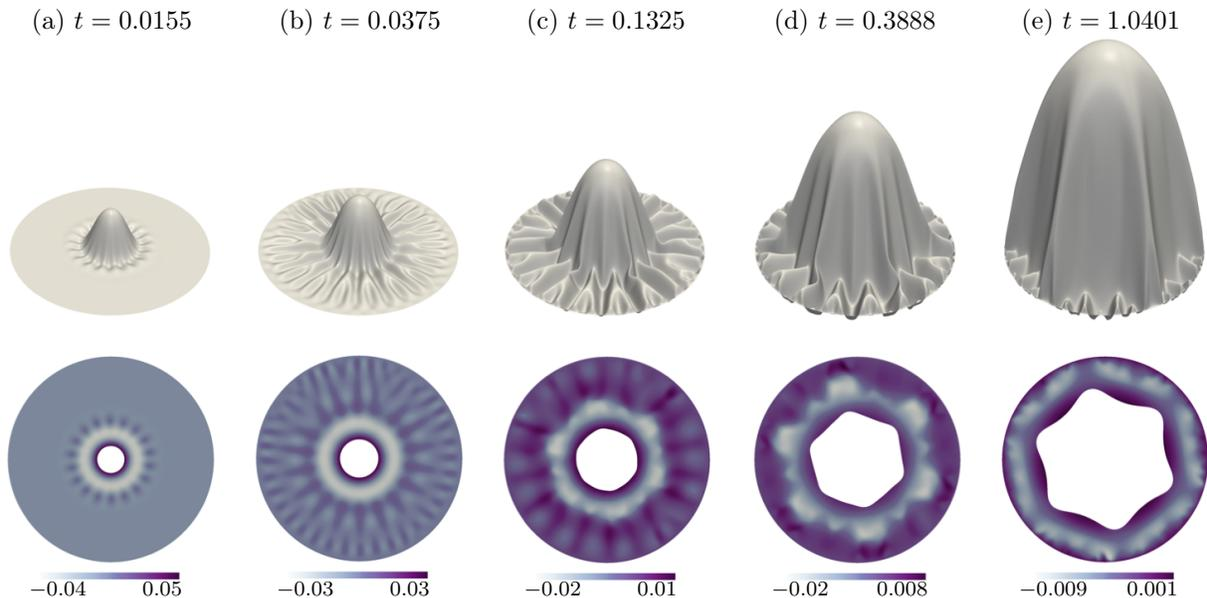
FIG. 9. Wrinkling excites fingering: time evolution of the air-liquid interface, the corresponding instantaneous pressure fields in the viscous fluid and the sheet deformations (with the transverse displacement increased by a factor of 10) for  $\mathcal{I} = 10^6$ .
