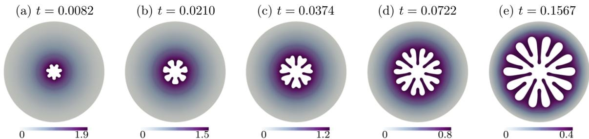
FIG. 4. Rigid cell: time evolution of the air-liquid interface and the corresponding instantaneous pressure field in the viscous fluid for  $\mathcal{I} = 0$ .
