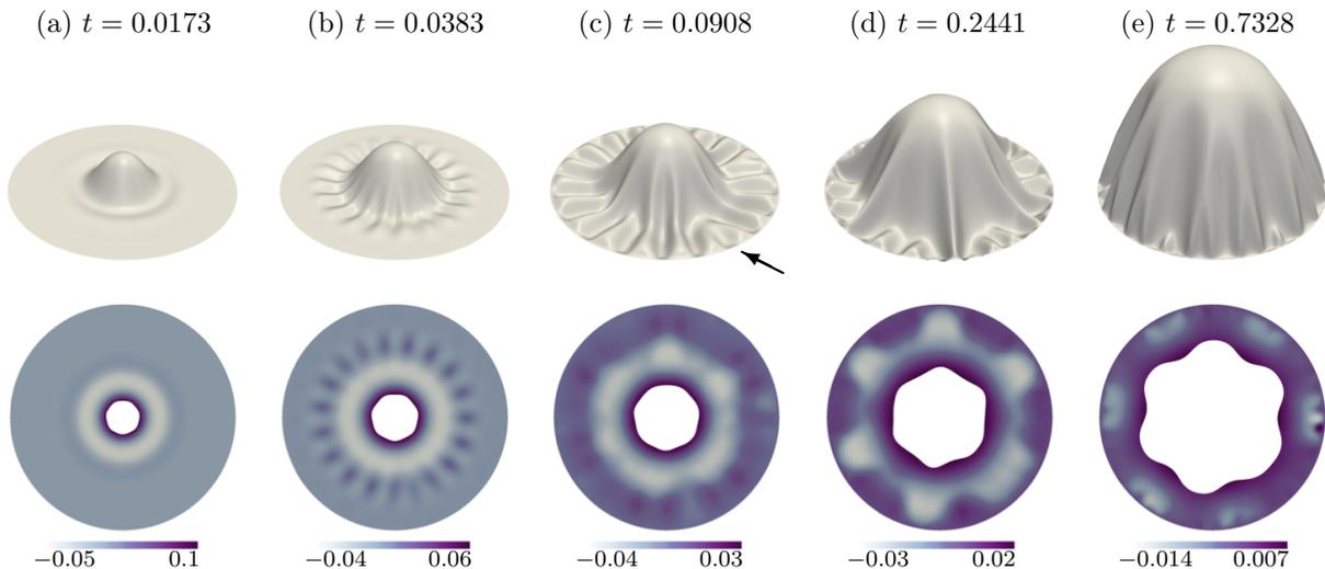
FIG. 8. Wrinkling alters fingering: time evolution of the air-liquid interface, the corresponding instantaneous pressure fields in the viscous fluid and the sheet deformations (with the transverse displacement increased by a factor of 10) for  $\mathcal{I} = 10^5$ . The arrow indicates the region of the small-scale frustration in the pattern.
