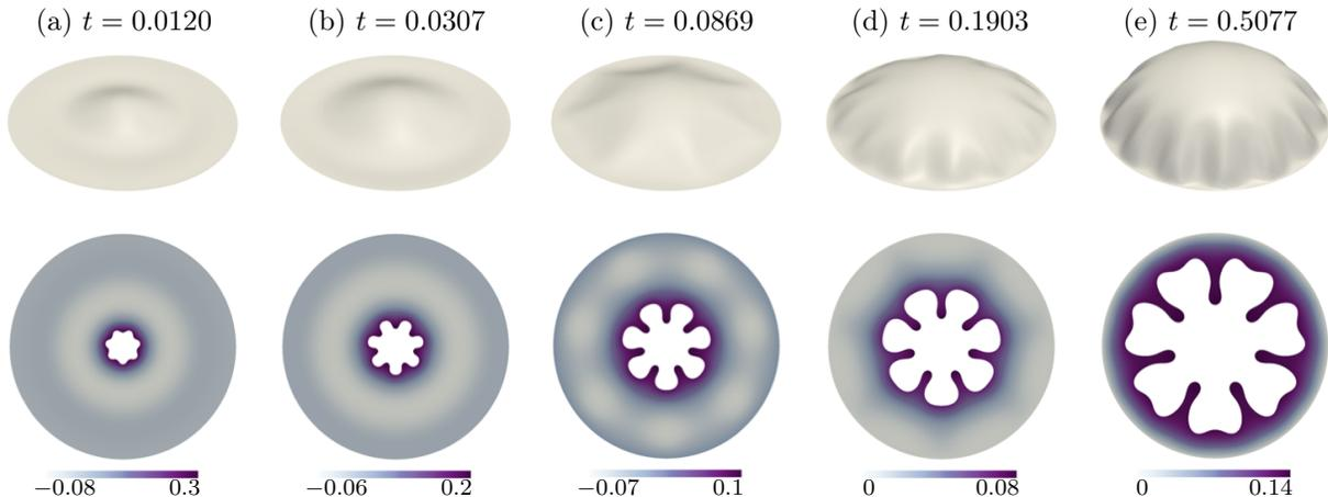
FIG. 6. Passive buckling: time evolution of the air-liquid interface, the corresponding instantaneous pressure fields in the viscous fluid and the sheet deformations (with the transverse displacement increased by a factor of 10) for  $\mathcal{I} = 10^3$ .
