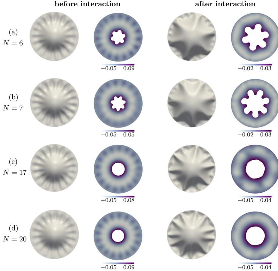
FIG. 10. Top view of the instantaneous sheet deformations and corresponding positions of the air-liquid interface and the pressure fields in the viscous fluid for  $\mathcal{I} = 10^4$ , before and after the interaction between wrinkling and fingering if the interface is perturbed at  $t = 0$  with (a)  $N = 6$ , (b)  $N = 7$ , (c)  $N = 17$  and (d)  $N = 20$ .
