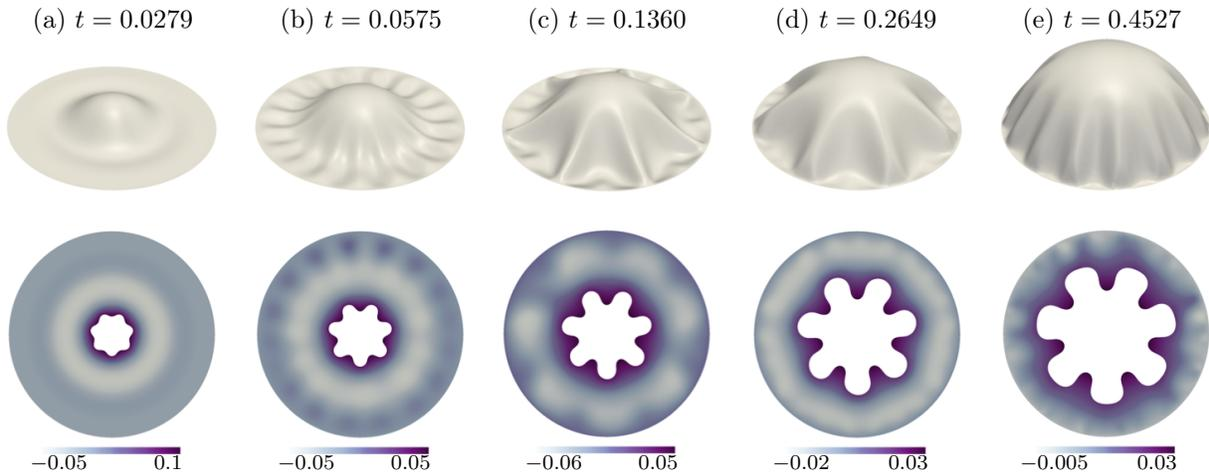
FIG. 7. Fingering controls wrinkling: time evolution of the air-liquid interface, the corresponding instantaneous pressure fields in the viscous fluid and the sheet deformations (with the transverse displacement increased by a factor of 10) for  $\mathcal{I} = 10^4$ .
